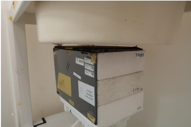
Bottom of Laptop, Test Separation 11 mm
