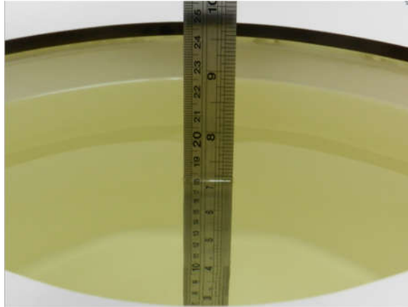
Fig 10.1 Photo of Liquid Height for Body SAR
