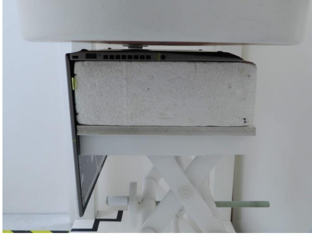
Bottom of Laptop, Test Separation 10 mm
