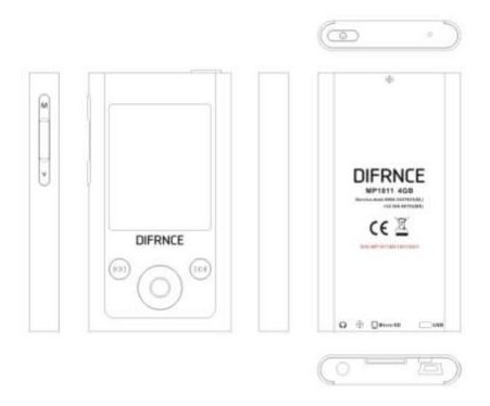
**M** key: refers to the Menu key. The menu will pop up after pressing this key, and then enter the next interface after confirming (Enter or Exit). Hold the key to go back to the main interface.
