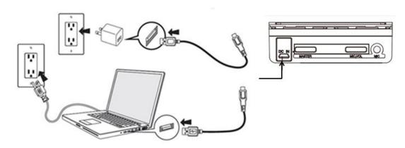
Note: When charging the unit for the first time, charge it for more than 12 hours to ensure you have a FULL initial charge.
