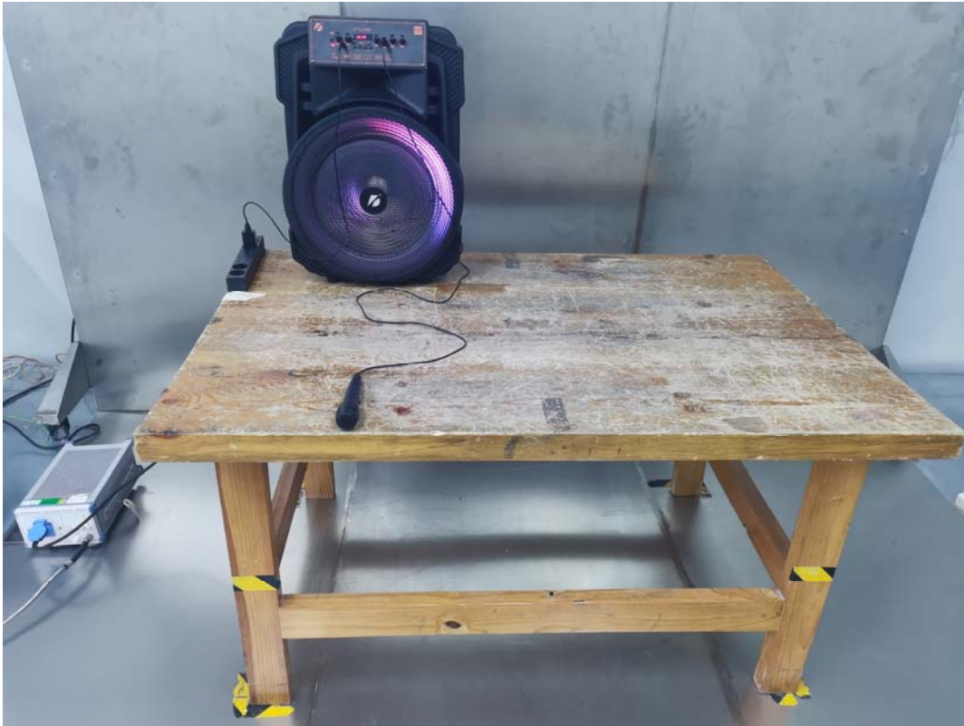
Conducted Emissions Side View- Power by USB port
