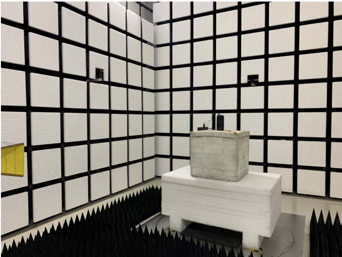
Radiated Emission Above 1GHz View
