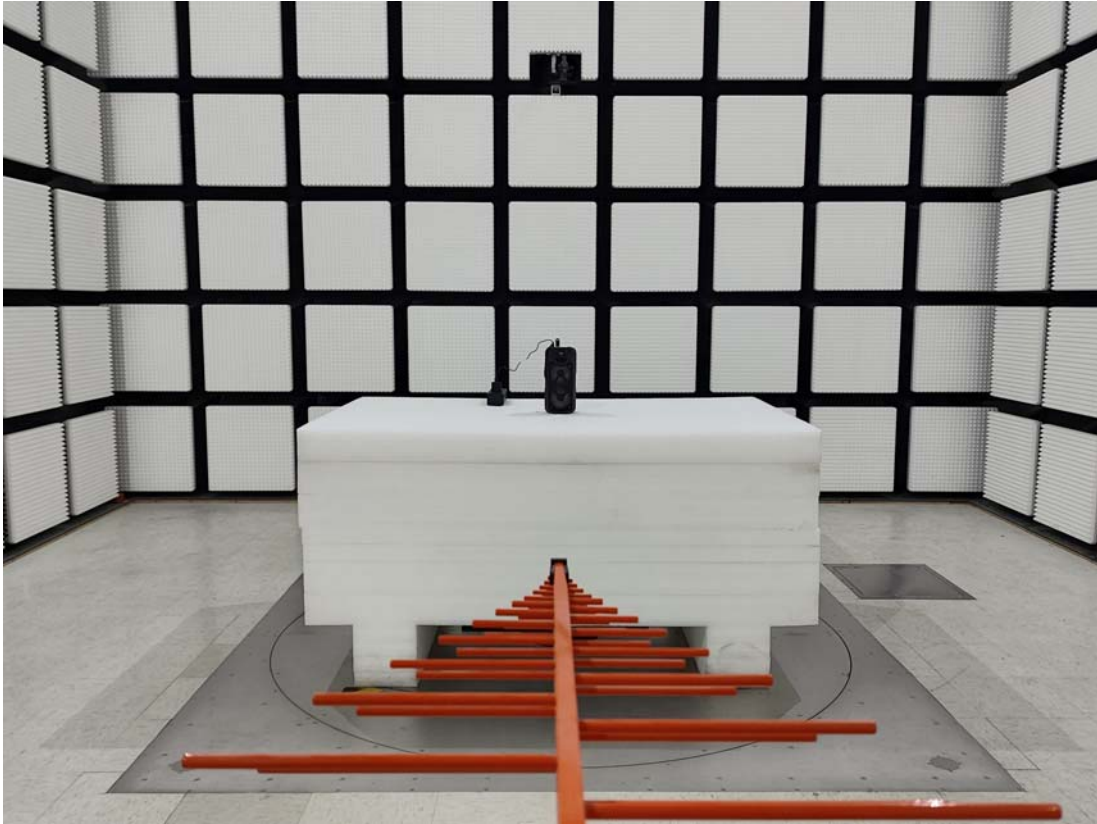
Radiated Emission Above 1GHz View
