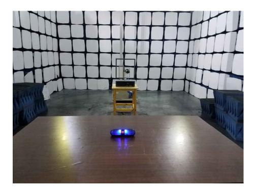
Radiation Emission Test Setup (30MHz to 1GHz)
