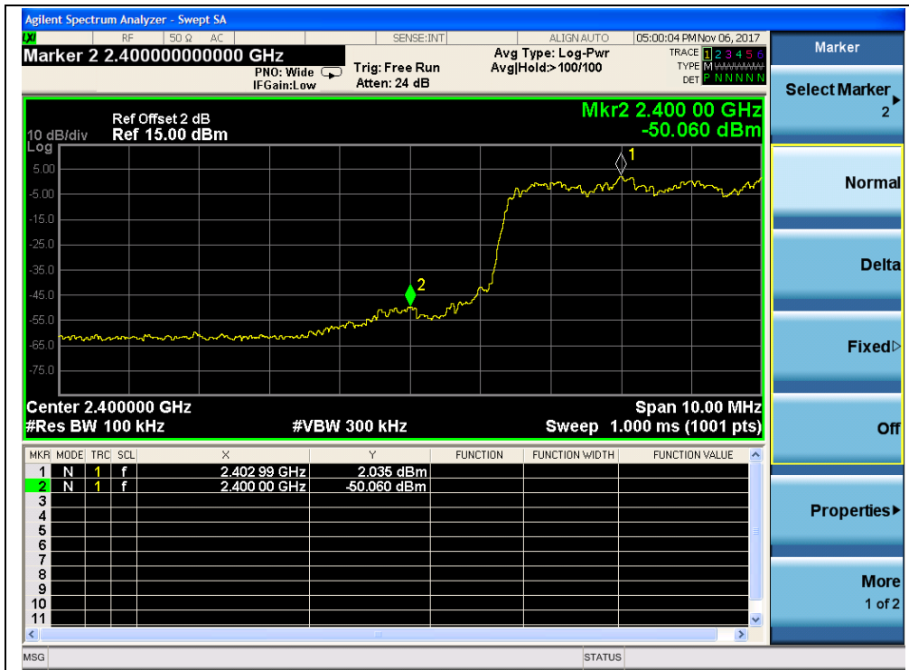
(Channel = 0, Band edge with hopping on @ 8-DPSK)
