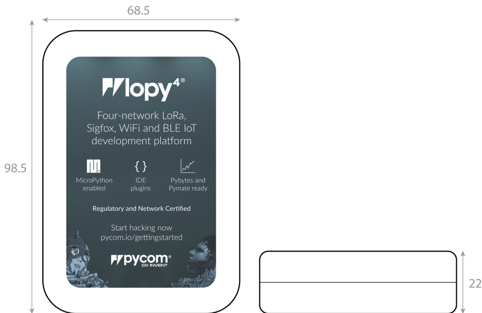
Figure 10 – Mechanical drawing of packaging – Units: mm
