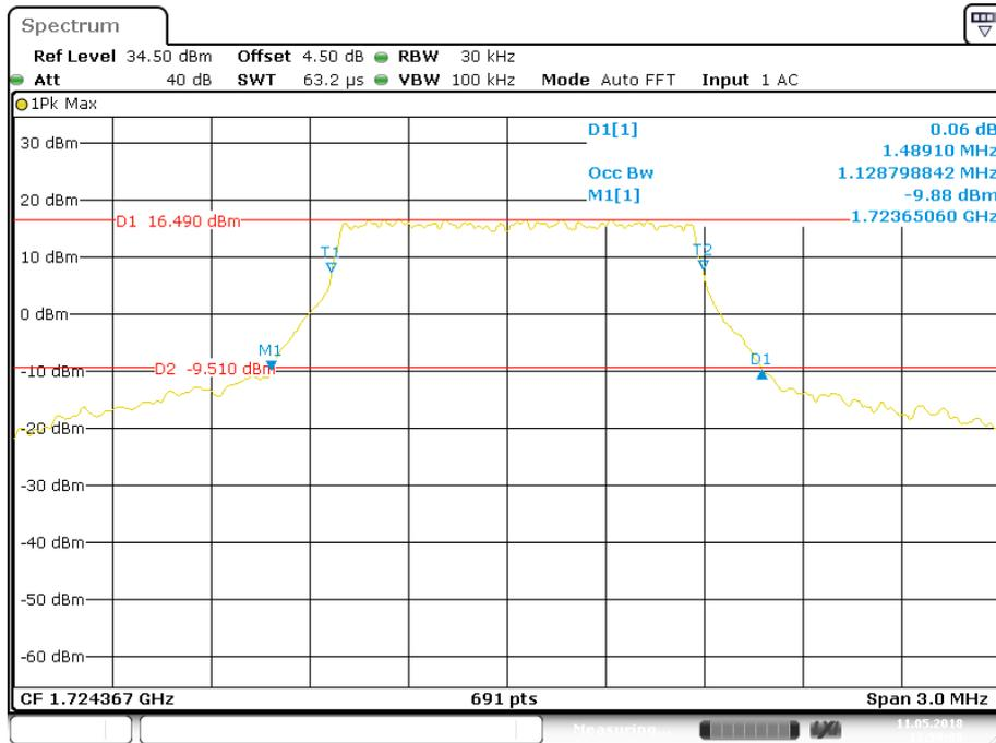
**16-QAM (20.0 MHz) - 26 dB Bandwidth & 99% Occupied Bandwidth, Middle channel**
