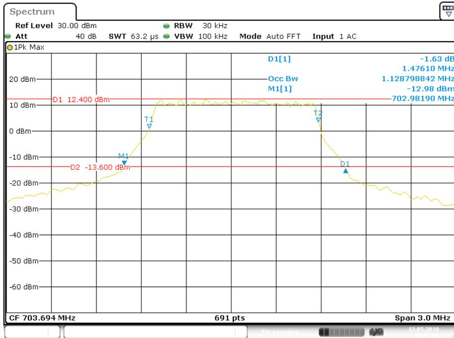
**16-QAM (10.0 MHz) - 26 dB Bandwidth & 99% Occupied Bandwidth, Middle channel**
