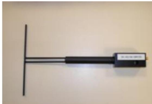
Figure 1 – Satimo COMOSAR Validation Dipole
