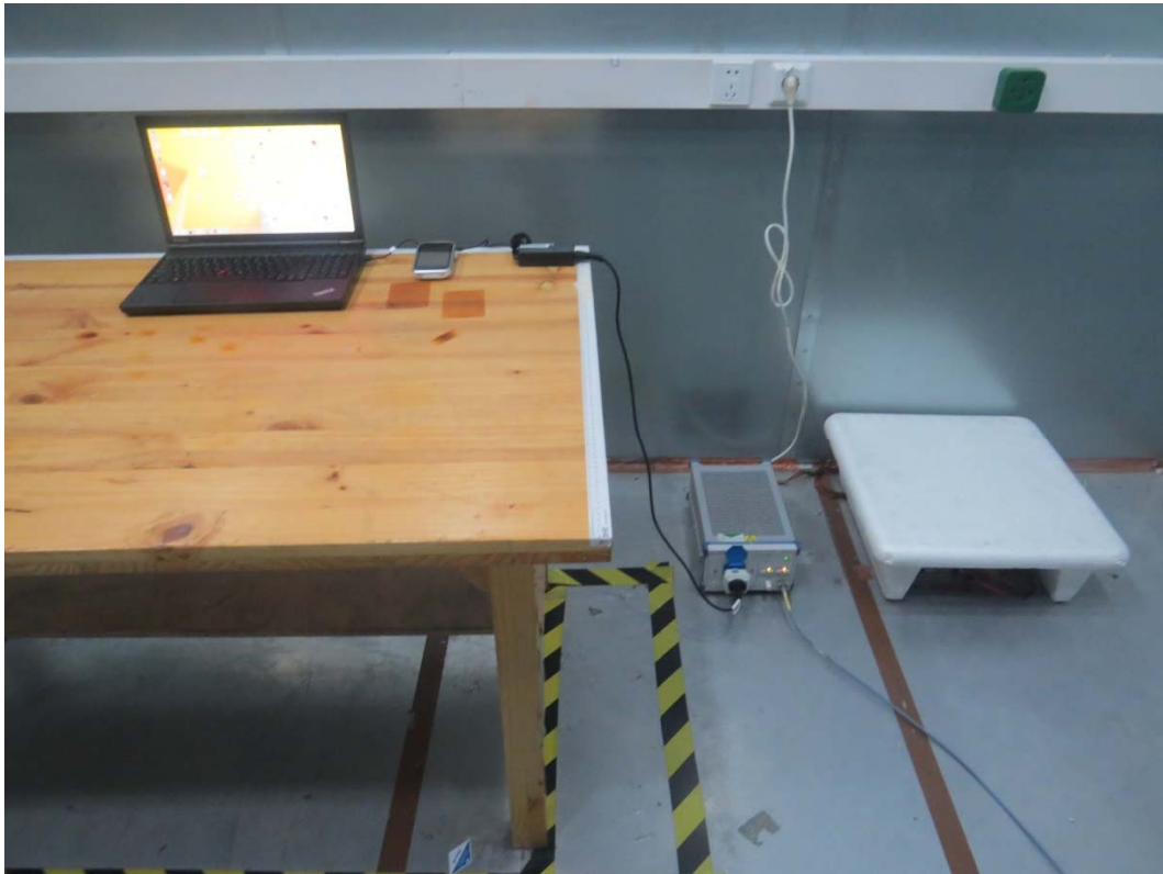
Picture 3 Conducted Emission Test Setup
