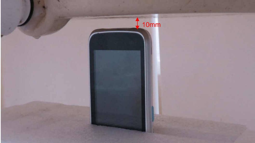
Picture10: Bottom Side, the distance from handset to the bottom of the Phantom is 10mm
