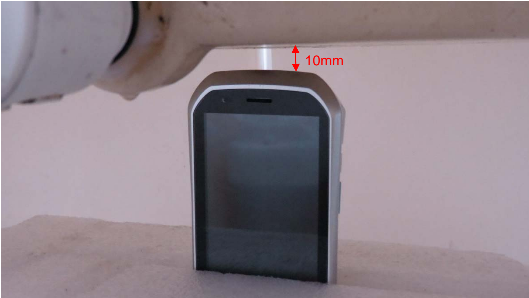
Picture9: Top Side, the distance from handset to the bottom of the Phantom is 10mm
