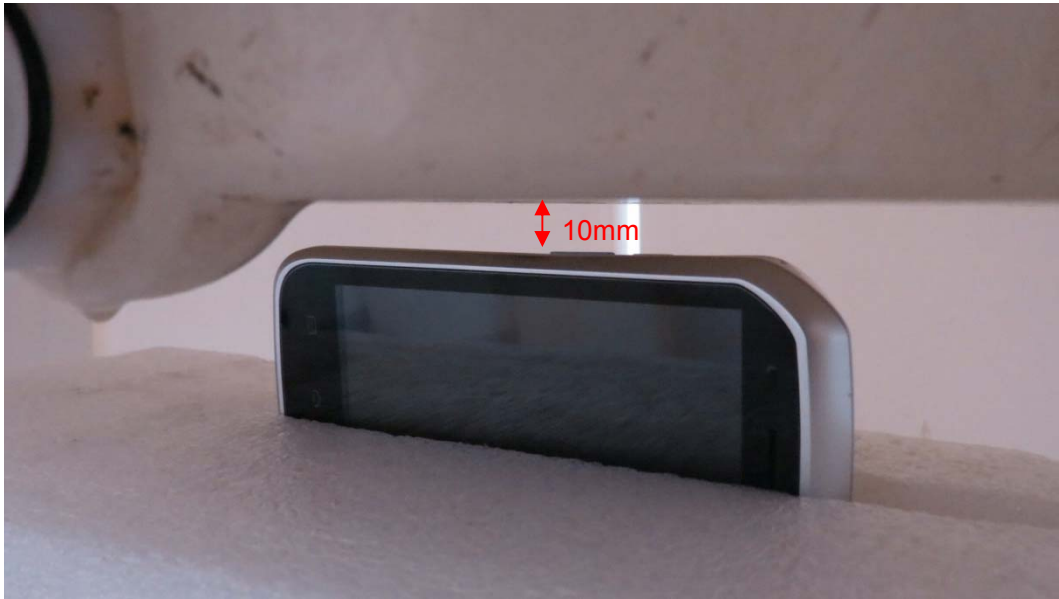
Picture16: Left Side, the distance from handset to the bottom of the Phantom is 10mm
