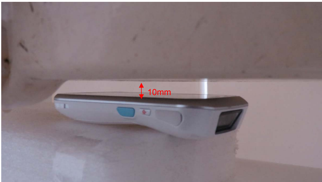
Picture15: Front Side, the distance from handset to the bottom of the Phantom is 10mm
