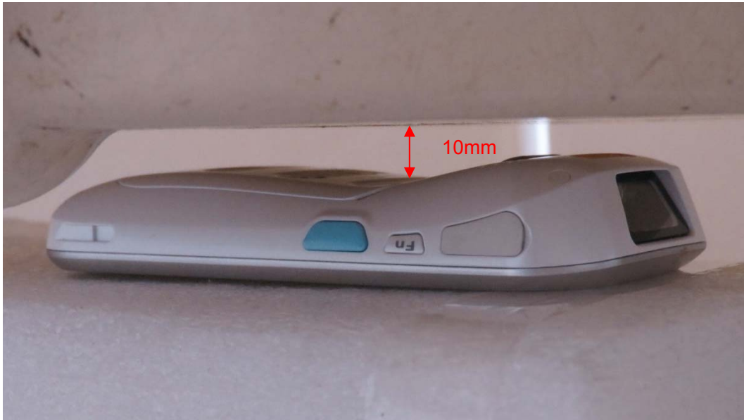
Picture14: Back Side, the distance from handset to the bottom of the Phantom is 10mm
