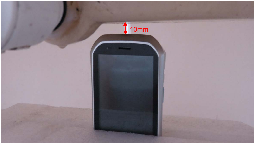
Picture18: Top Side, the distance from handset to the bottom of the Phantom is 10mm
