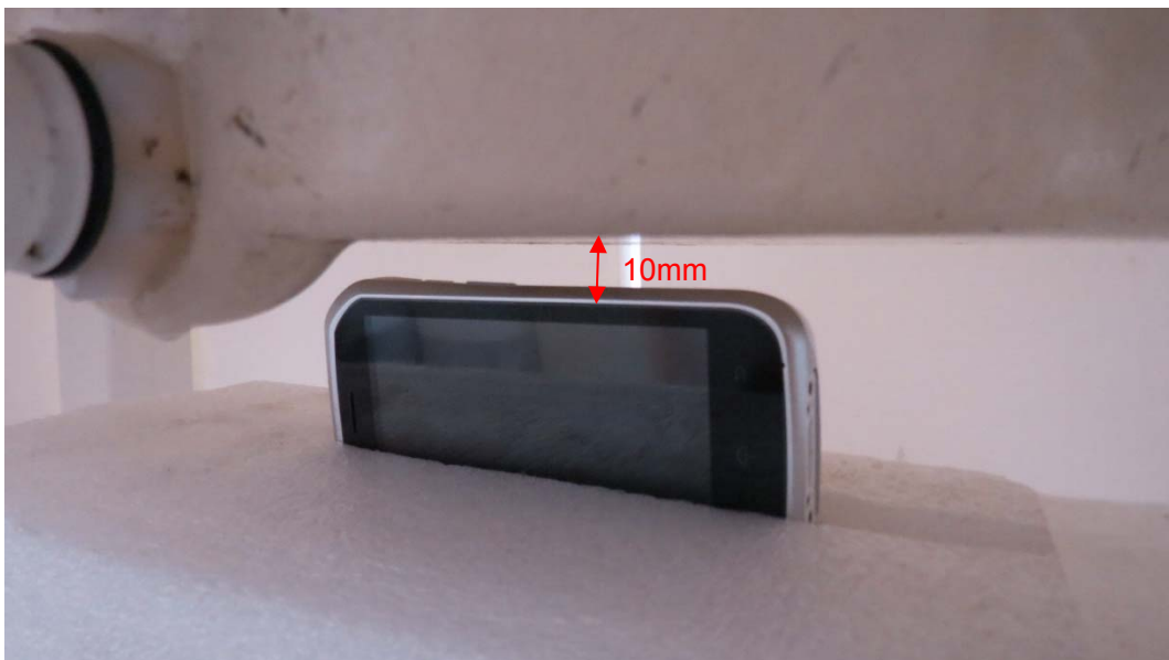
Picture17: Right Side, the distance from handset to the bottom of the Phantom is 10mm
