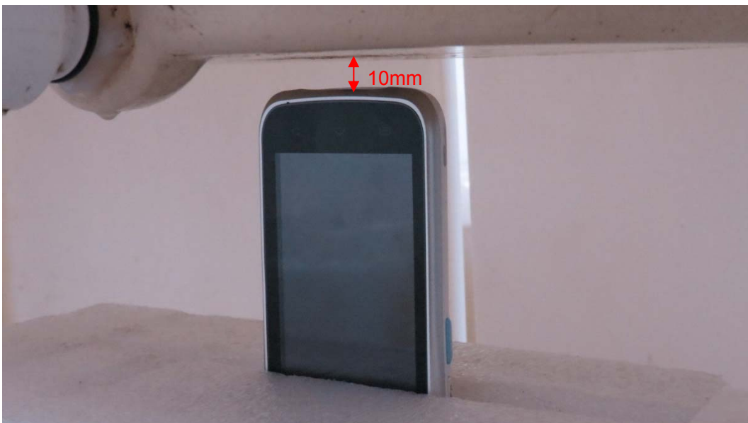
Picture19: Bottom Side, the distance from handset to the bottom of the Phantom is 10mm
