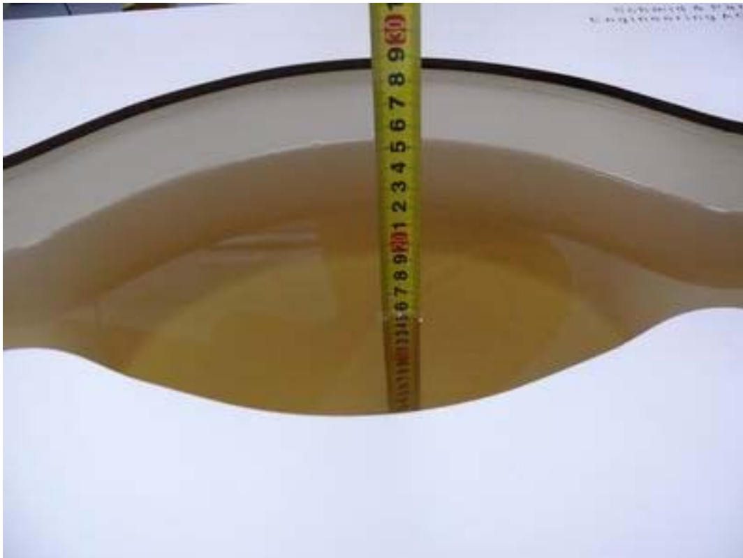
Picture4: Liquid depth in the flat Phantom (835MHz, 15.4cm depth)
