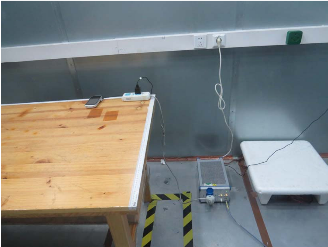
Picture 3 Conducted Emission Test Setup
