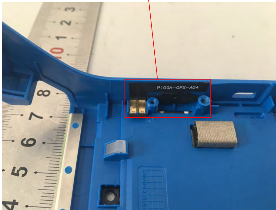
EUT – BT&2.4G WIFI Antenna View
