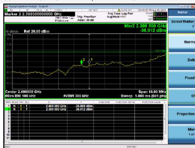
802.11b HIGH CHANNEL, BAND EDGE
