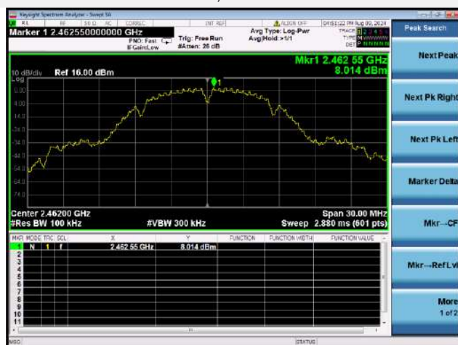
802.11b HIGH CHANNEL, CARRIER LEVEL
