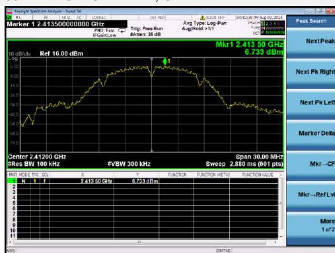
802.11b HIGH CHANNEL, CARRIER LEVEL
