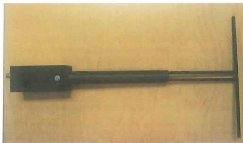
Figure 1 – MVG COMOSAR Validation Dipole
