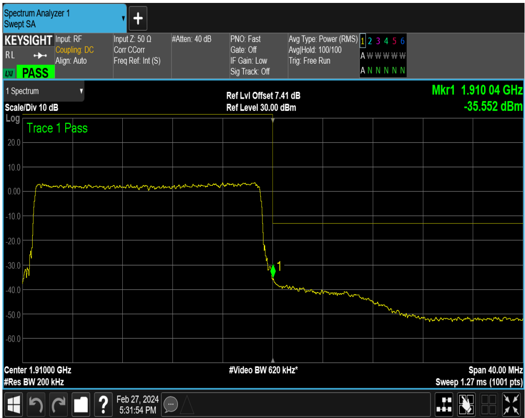
Band2 QPSK BW=3MHz Channel=18615 RB Size=15 Position=#0
