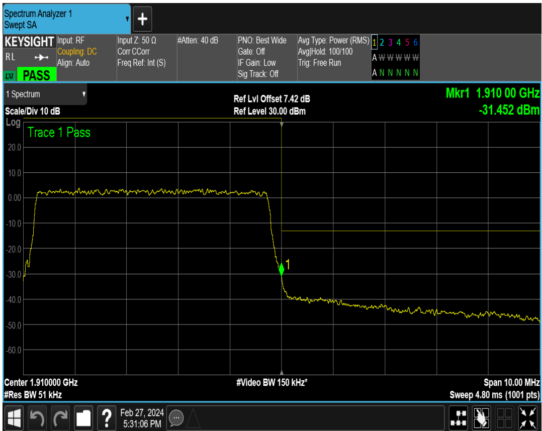
Band2 QPSK BW=5MHz Channel=19175 RB Size=25 Position=#0
