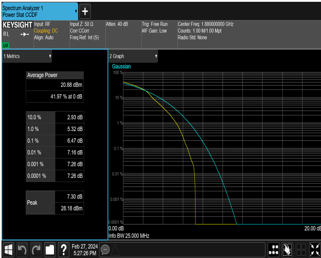
Band2 QAM16 BW=10MHz Channel=18900 RB Size=1 Position=#0
