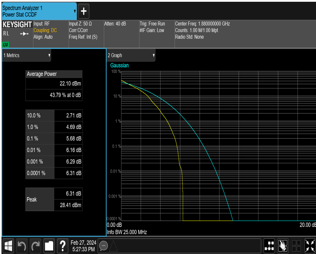
Band2 QAM16 BW=15MHz Channel=18900 RB Size=1 Position=#0
