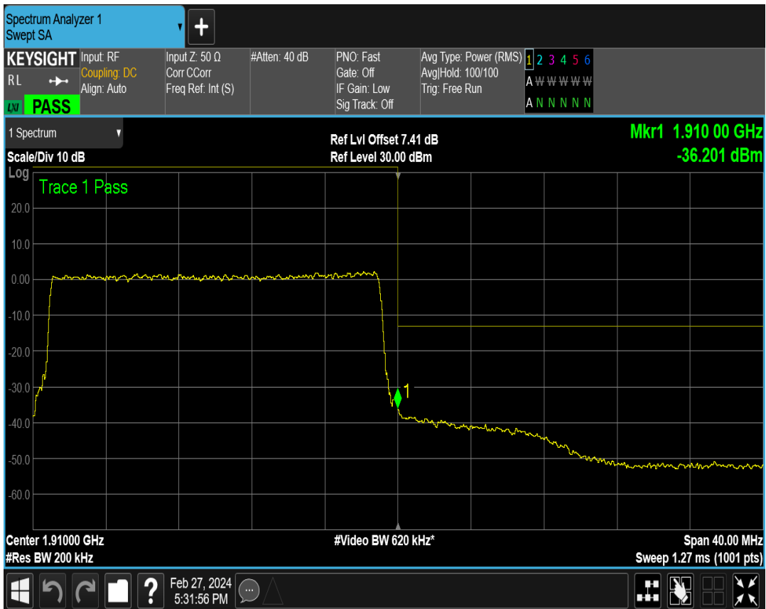
Band2 QAM16 BW=3MHz Channel=18615 RB Size=15 Position=#0
