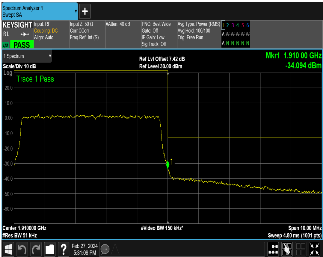
Band2 QPSK BW=1.4MHz Channel=18607 RB Size=6 Position=#0
