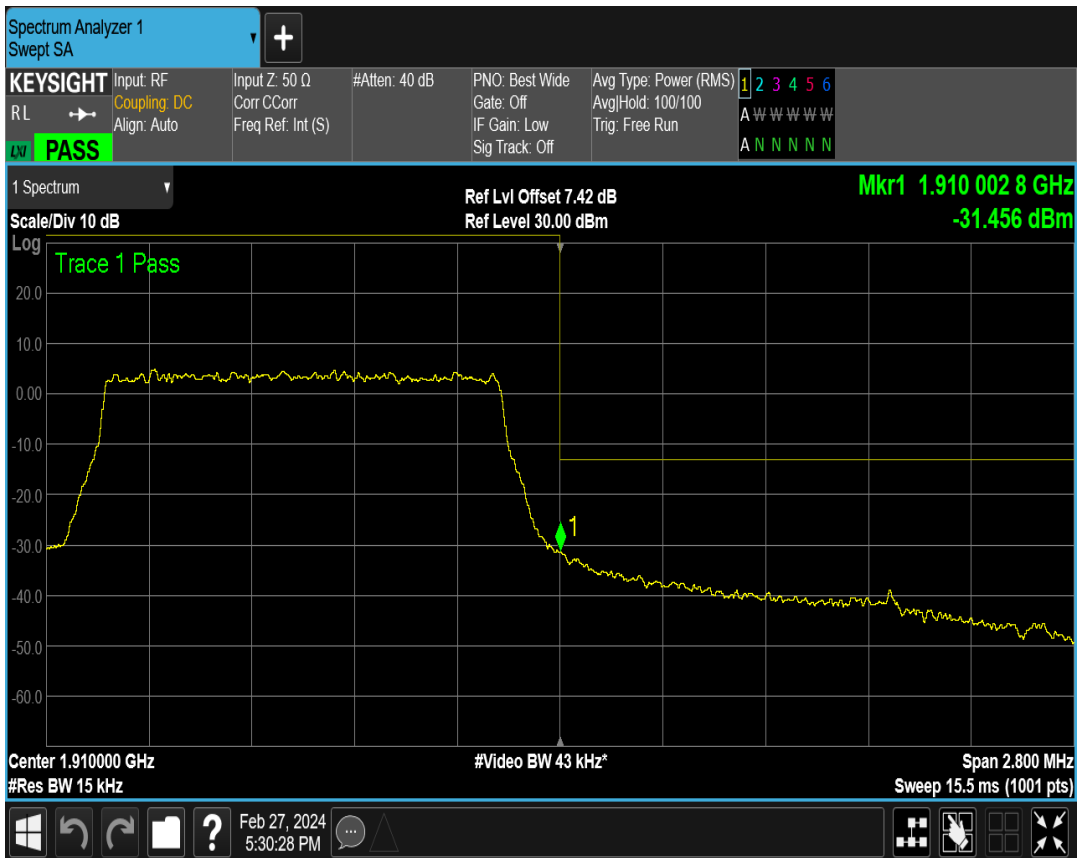
Band2 QPSK BW=10MHz Channel=18650 RB Size=50 Position=#0
