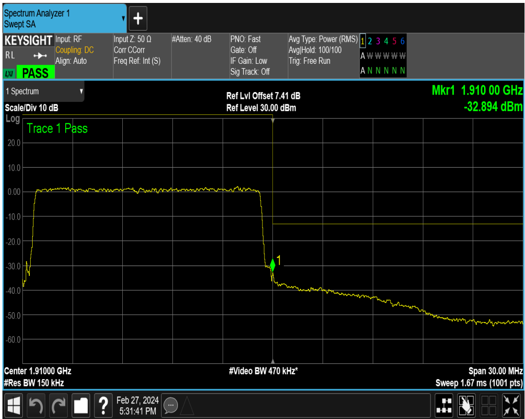
Band2 QAM16 BW=20MHz Channel=18700 RB Size=100 Position=#0
