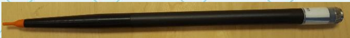
Figure 2 – MVG COMOSAR Dosimetric E field Dipole
