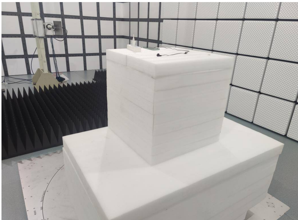
Photo of Radiated Emission Measurement (Above 1G)
