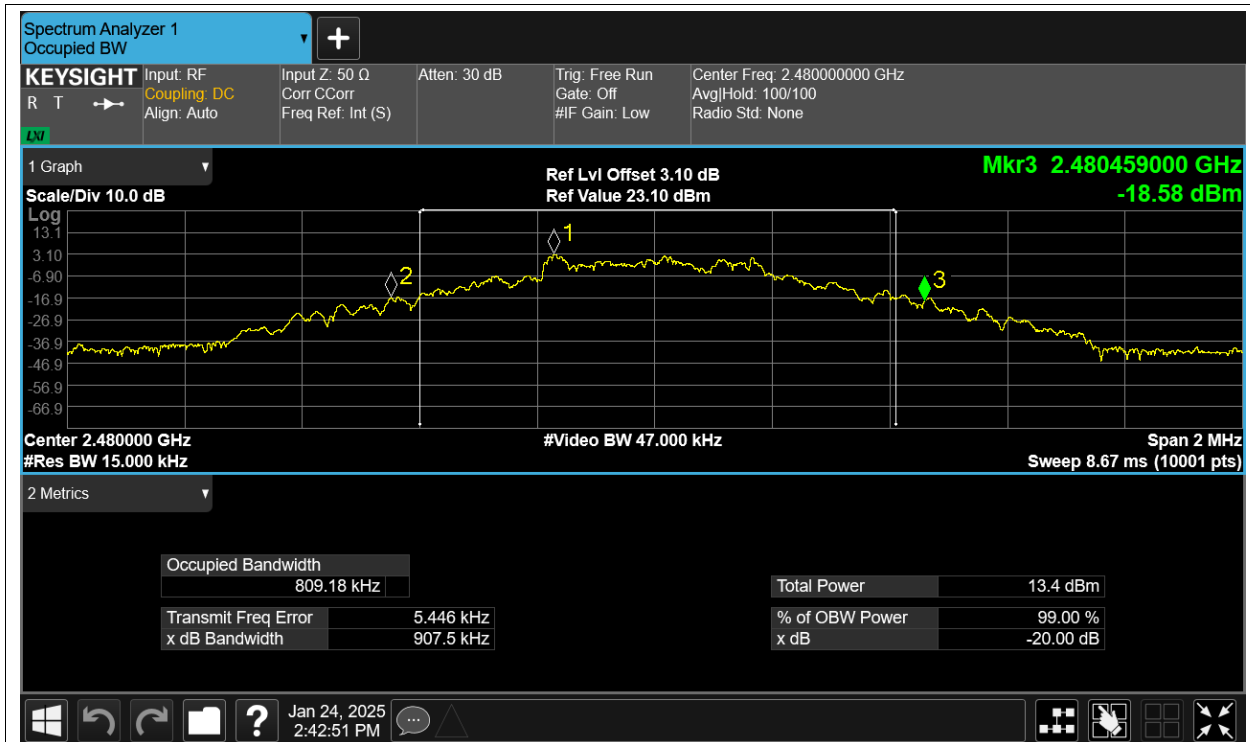
-20dB Bandwidth NVNT 2-DH1 2402MHz Ant1
