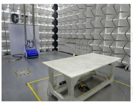
Radiated spurious emission Test Setup-2(30M-1G)
