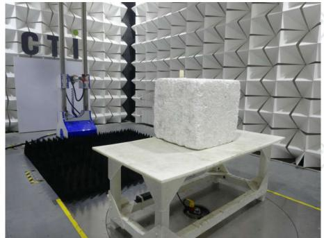
Radiated spurious emission Test Setup-3(Above 1GHz)
