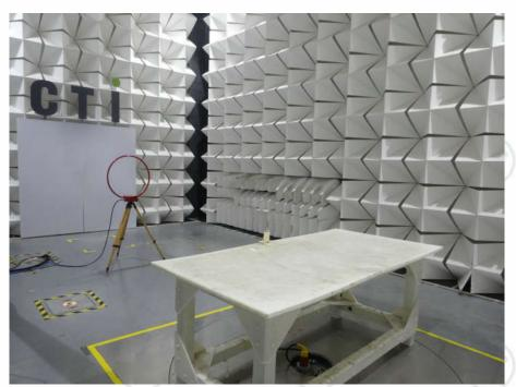
Radiated spurious emission Test Setup-1(9k-30M)
