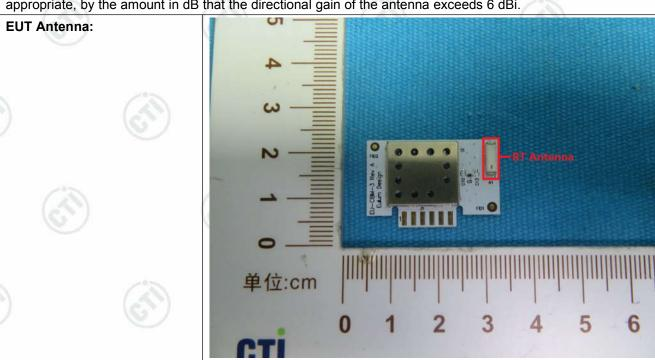
The antenna is chip Antenna and no consideration of replacement. The best case gain of the antenna is 1.3dBi.
