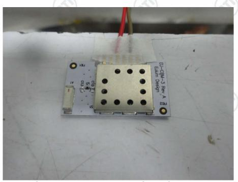
Conducted Emissions Test Setup(Close up)
