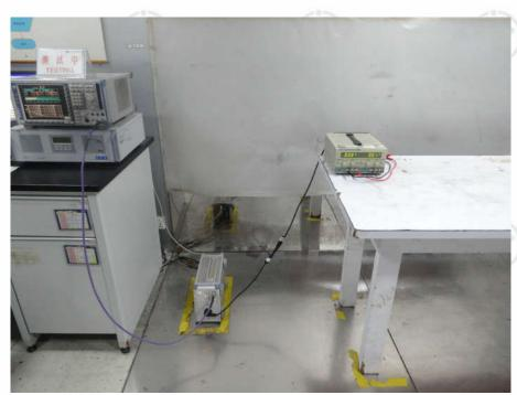
**Conducted Emissions Test Setup**
