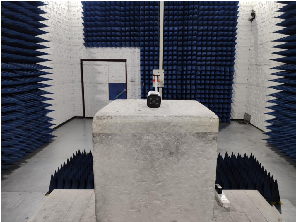
FCC RADIATED EMISSION TEST SETUP ABOVE 1GHZ
