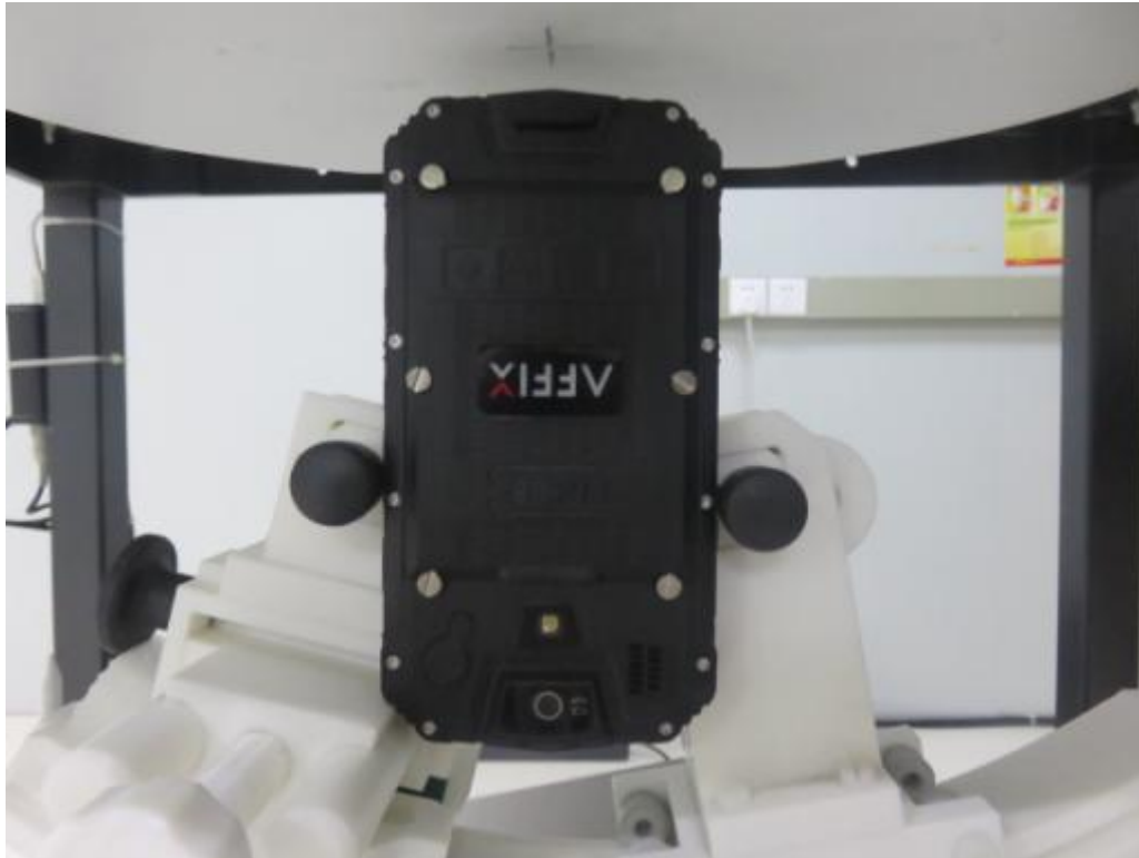
10mm body-worn Bottom Side Setup Photo(hotspot)
