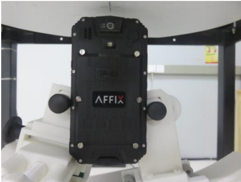
10mm body-worn Top Side Setup Photo(hotspot)
