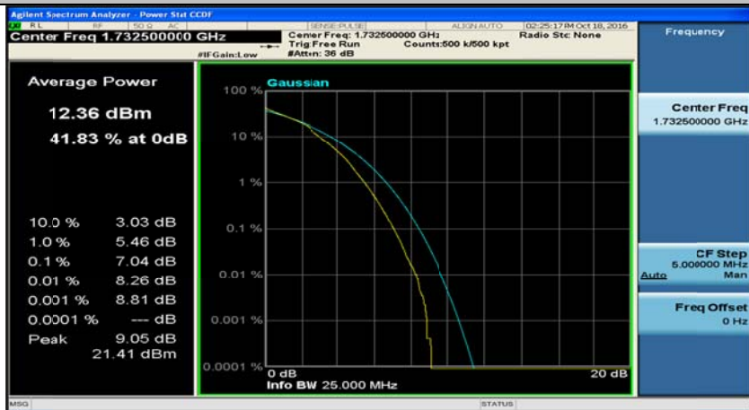
(Channel Bandwidth:15 MHz)_MCH_16QAM_75RB#0
