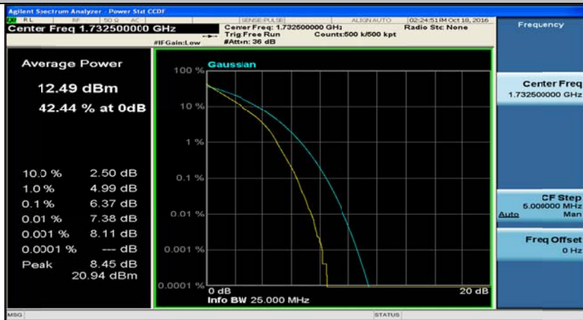
(Channel Bandwidth:15 MHz)_MCH_QPSK_37RB#38
