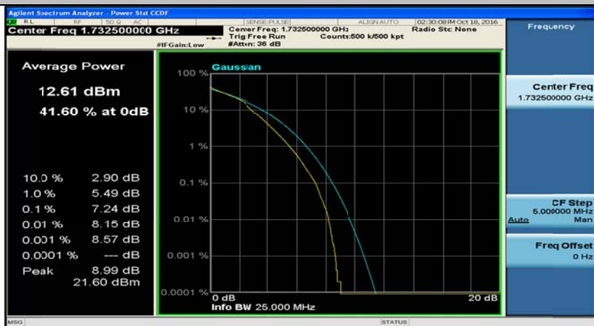
(Channel Bandwidth:20 MHz)_MCH_16QAM_50RB#50
