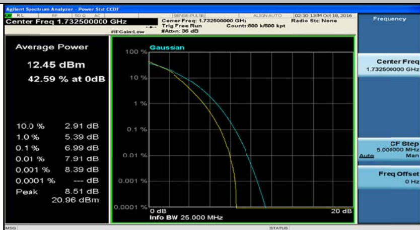
(Channel Bandwidth:20 MHz)_MCH_16QAM_100RB#0
