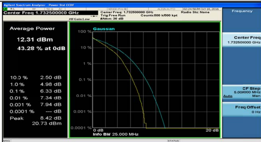
(Channel Bandwidth:15 MHz)_MCH_QPSK_75RB#0
