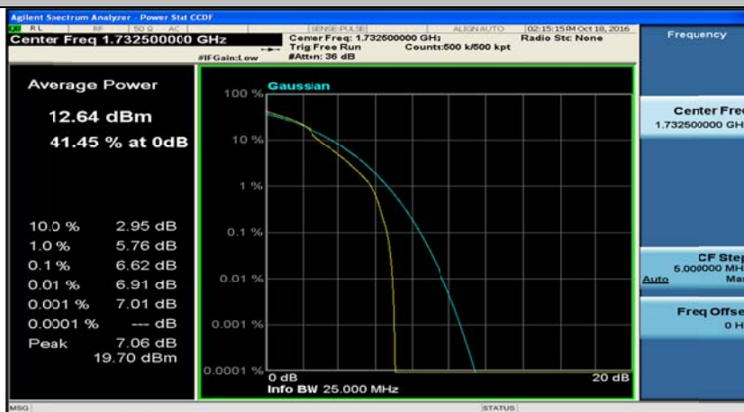
(Channel Bandwidth: 5 MHz)_MCH_16QAM_12RB#0
