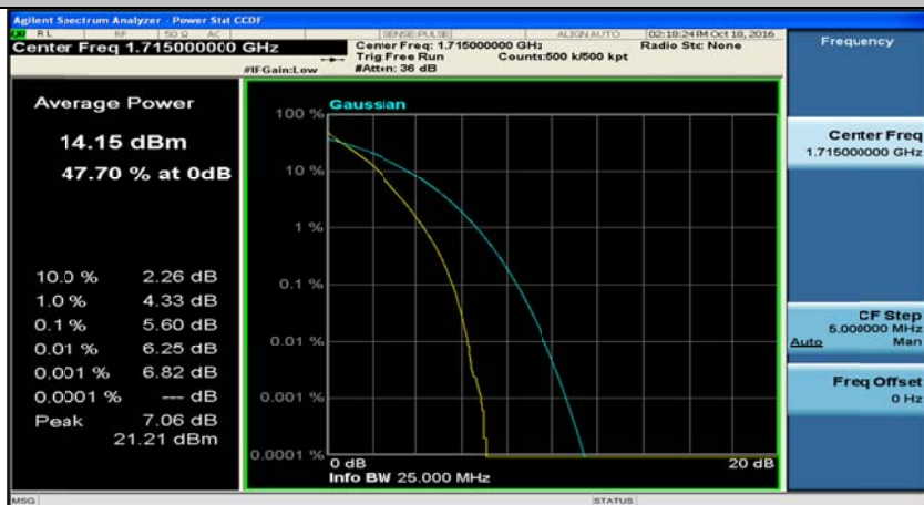
Channel Bandwidth: 10 MHz_LCH_QPSK_25RB#12
