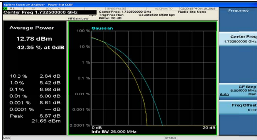
Channel Bandwidth: 10 MHz_MCH_16QAM_25RB#12
