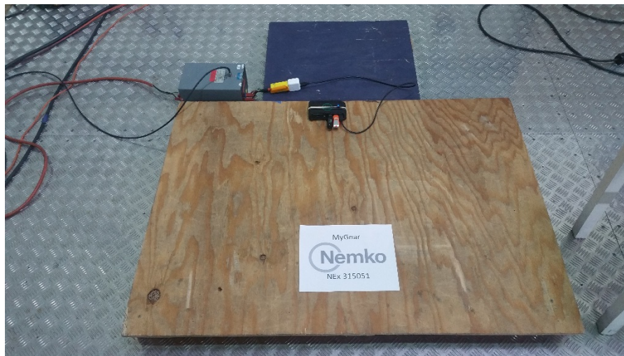
Figure 8.7-1: Clause 9.5 – Radio frequency, common mode setup photo
