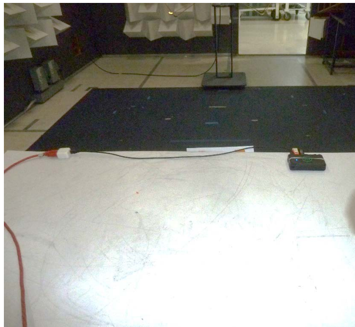
Figure 8.4-2: Clause 9.2 – Radio frequency electromagnetic field (0.8 to 1 and 1.4 to 2.7 GHz) setup photo
