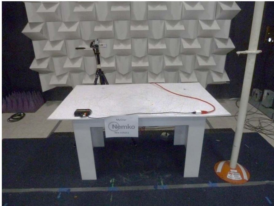
Figure 8.4-1: Clause 9.2 – Radio frequency electromagnetic field (0.8 to 1 and 1.4 to 2.7 GHz) setup photo
