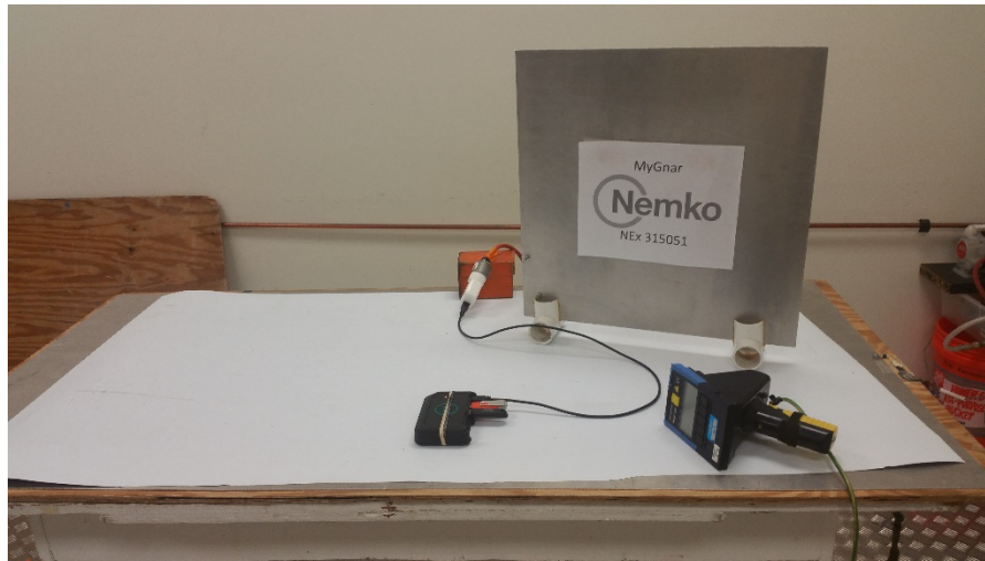
Figure 8.5-3: Clause 9.3 – Electrostatic discharge setup photo
