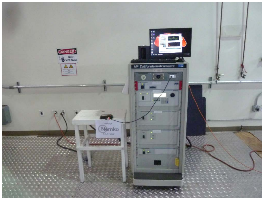
Figure 8.2-1: Clause 8.5 – Harmonic current emissions (AC mains input port) setup photo
