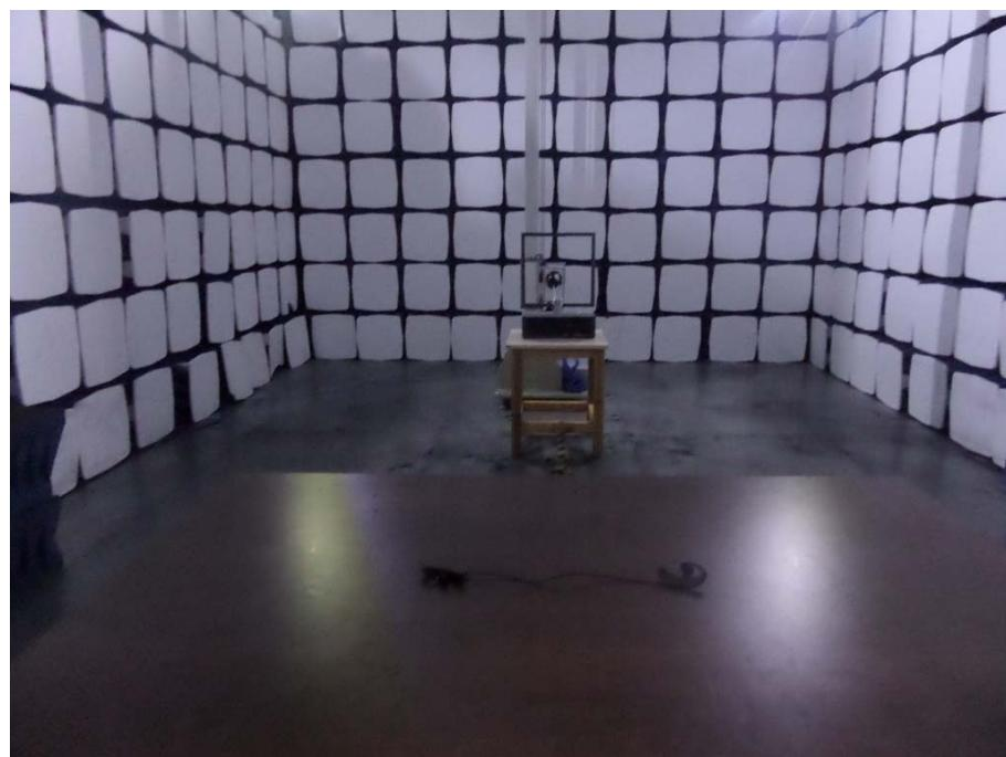
**Radiation Emission Test Setup (30MHz to 1GHz)**
