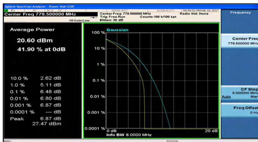
(LTE band 13_Channel Bandwidth: 5 MHz)_LCH_QPSK_12RB#13
