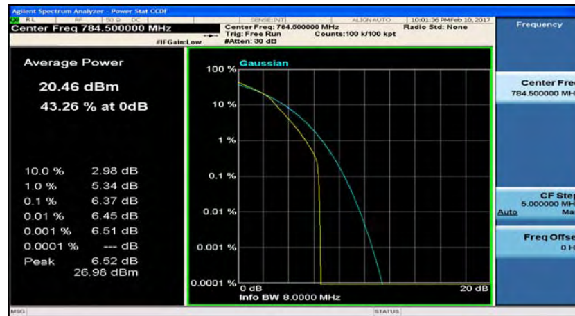
(LTE band 13_Channel Bandwidth: 5 MHz)_HCH_16QAM_12RB#6
