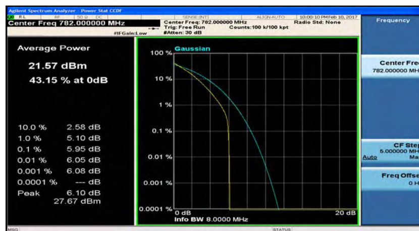
(LTE band 13_Channel Bandwidth: 5 MHz)_MCH_QPSK_12RB#13
