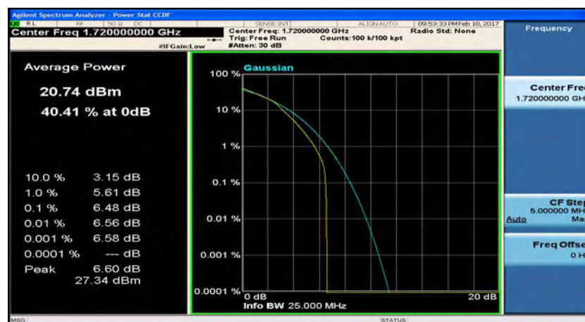
(LTE band 4_Channel Bandwidth:20 MHz)_LCH_16QAM_50RB#50
