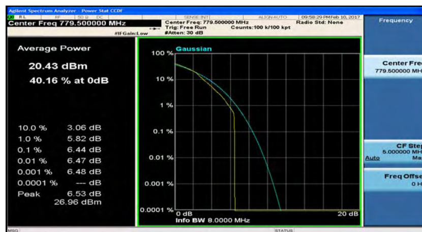
(LTE band 13_Channel Bandwidth: 5 MHz)_LCH_16QAM_1RB#12
