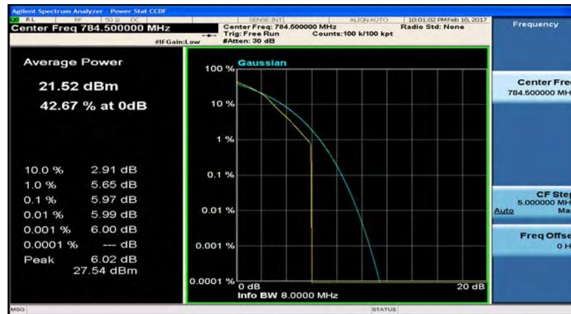
(LTE band 13_Channel Bandwidth: 5 MHz)_HCH_16QAM_1RB#12
