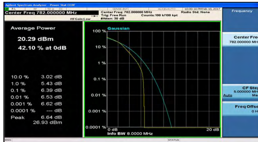
(LTE band 13_Channel Bandwidth: 5 MHz)_MCH_16QAM_12RB#6
