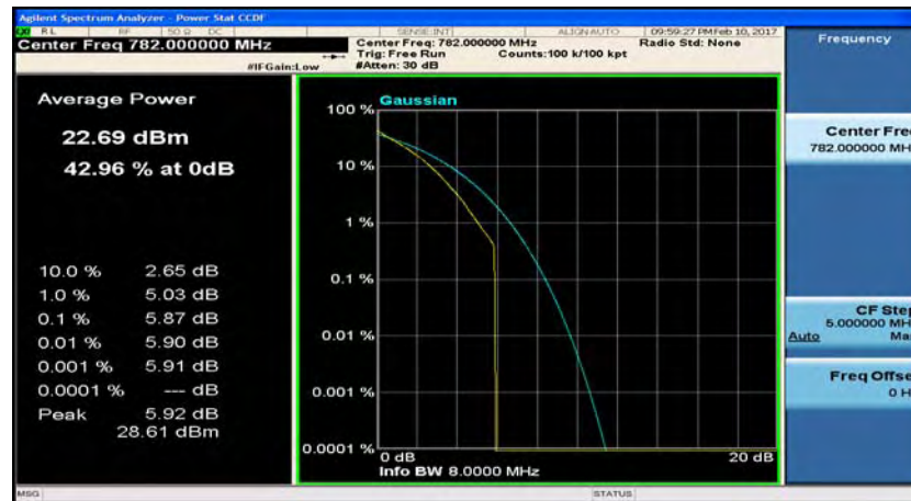
(LTE band 13_Channel Bandwidth: 5 MHz)_MCH_QPSK_1RB#12
