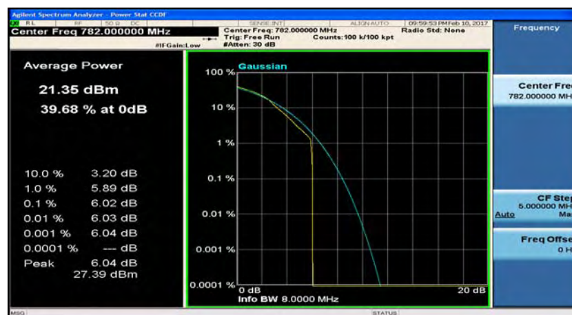
(LTE band 13_Channel Bandwidth: 5 MHz)_MCH_16QAM_1RB#24
