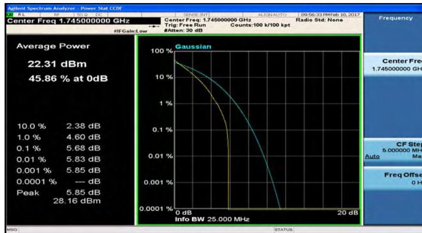
(LTE band 4_Channel Bandwidth:20 MHz)_HCH_QPSK_50RB#25
