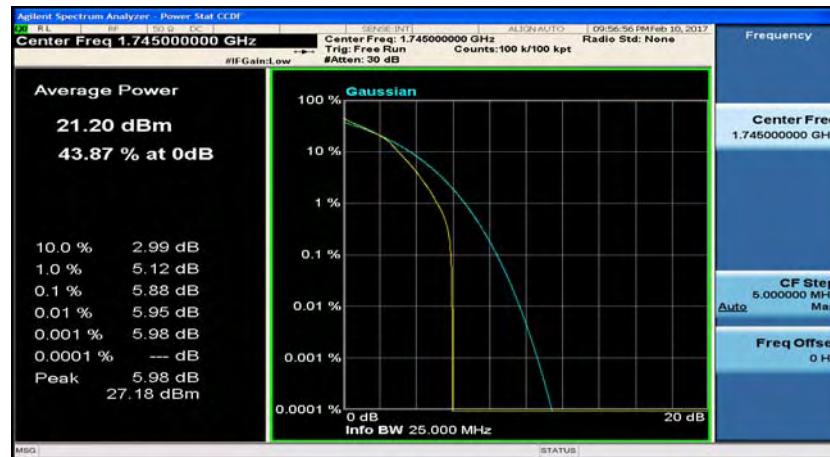
(LTE band 4_Channel Bandwidth:20 MHz)_HCH_16QAM_50RB#25
