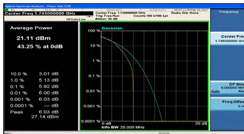
(LTE band 4_Channel Bandwidth:20 MHz)_HCH_16QAM_50RB#50
