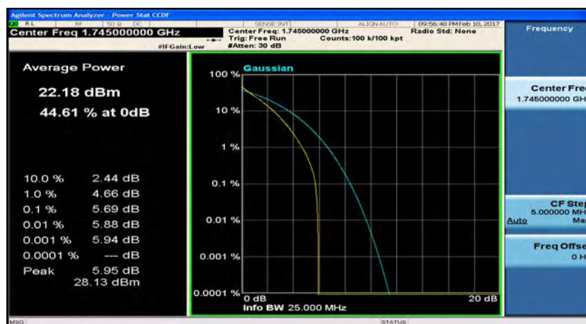
(LTE band 4_Channel Bandwidth:20 MHz)_HCH_QPSK_50RB#50
