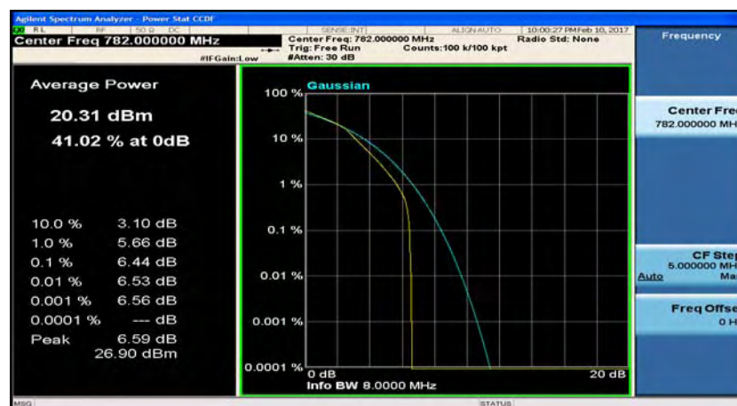
(LTE band 13_Channel Bandwidth: 5 MHz)_MCH_16QAM_12RB#13
