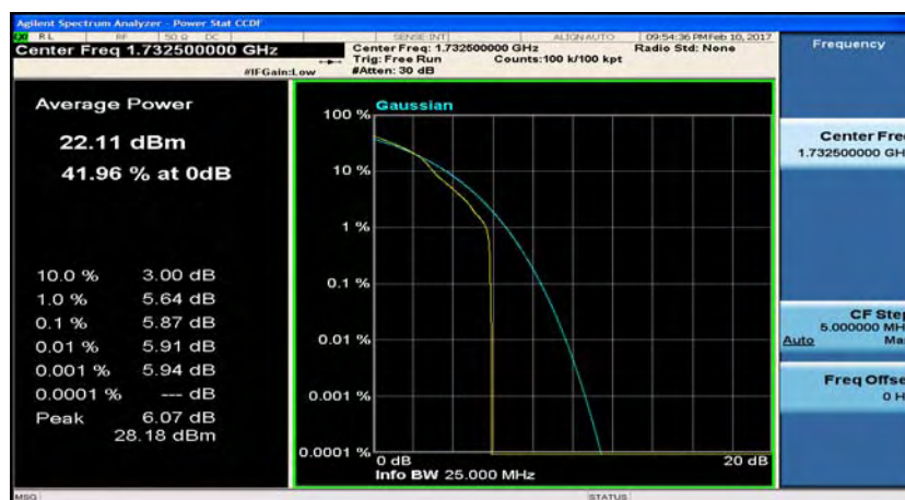
(LTE band 4_Channel Bandwidth:20 MHz)_MCH_16QAM_1RB#99
