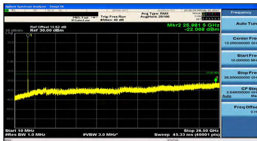
(LTE band 4_Channel Bandwidth: 5 MHz)_MCH_QPSK_1RB#24
