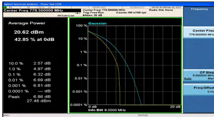
(LTE band 13_Channel Bandwidth: 5 MHz)_LCH_QPSK_12RB#6
