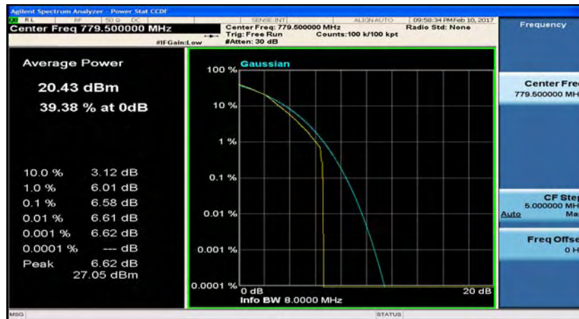
(LTE band 13_Channel Bandwidth: 5 MHz)_LCH_16QAM_12RB#0
