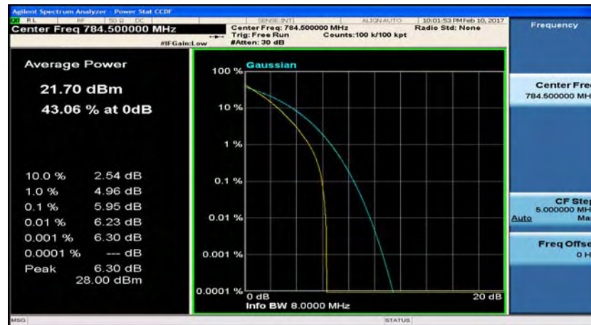
(LTE band 13_Channel Bandwidth: 5 MHz)_LCH_16QAM_1RB#0
