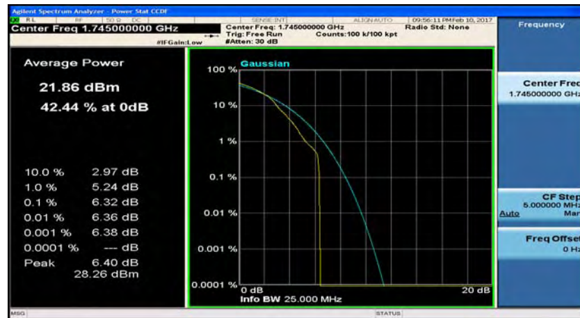
(LTE band 4_Channel Bandwidth:20 MHz)_HCH_16QAM_1RB#49
