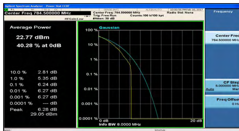
(LTE band 13_Channel Bandwidth: 5 MHz)_HCH_QPSK_1RB#24
