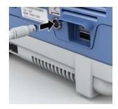
Push the cord connector into the foot switch port until the connector automatically makes a 1/4 turn and you hear a click sound.
