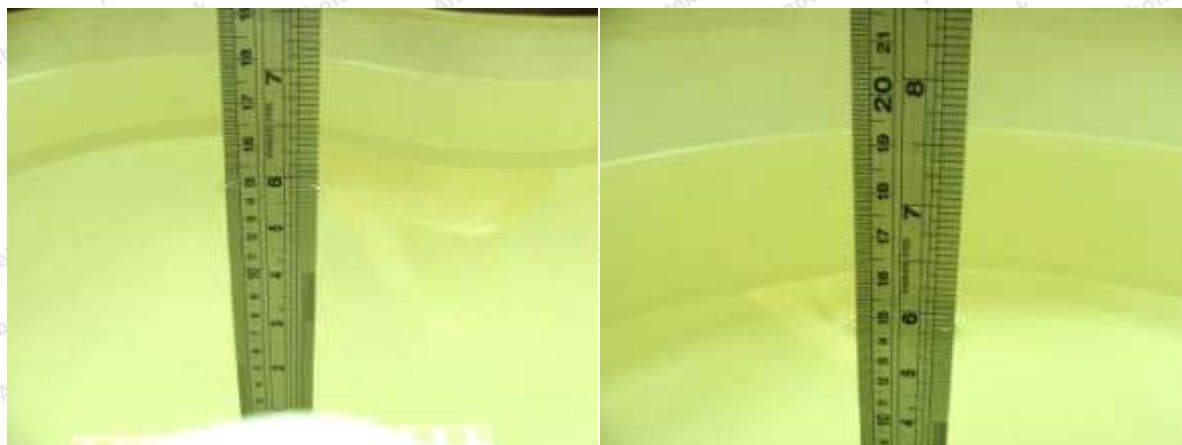
Photo of Liquid Height for Head SAR
