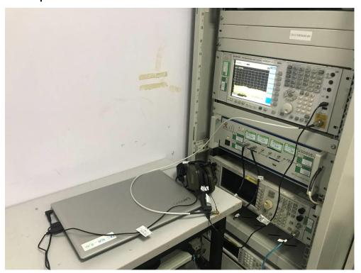
Conducted Emissions at AC Power Line (150kHz-30MHz)
