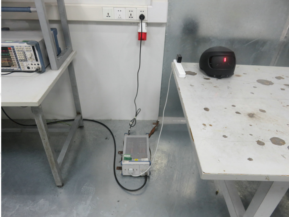
Photo of Conducted Emission Measurement
