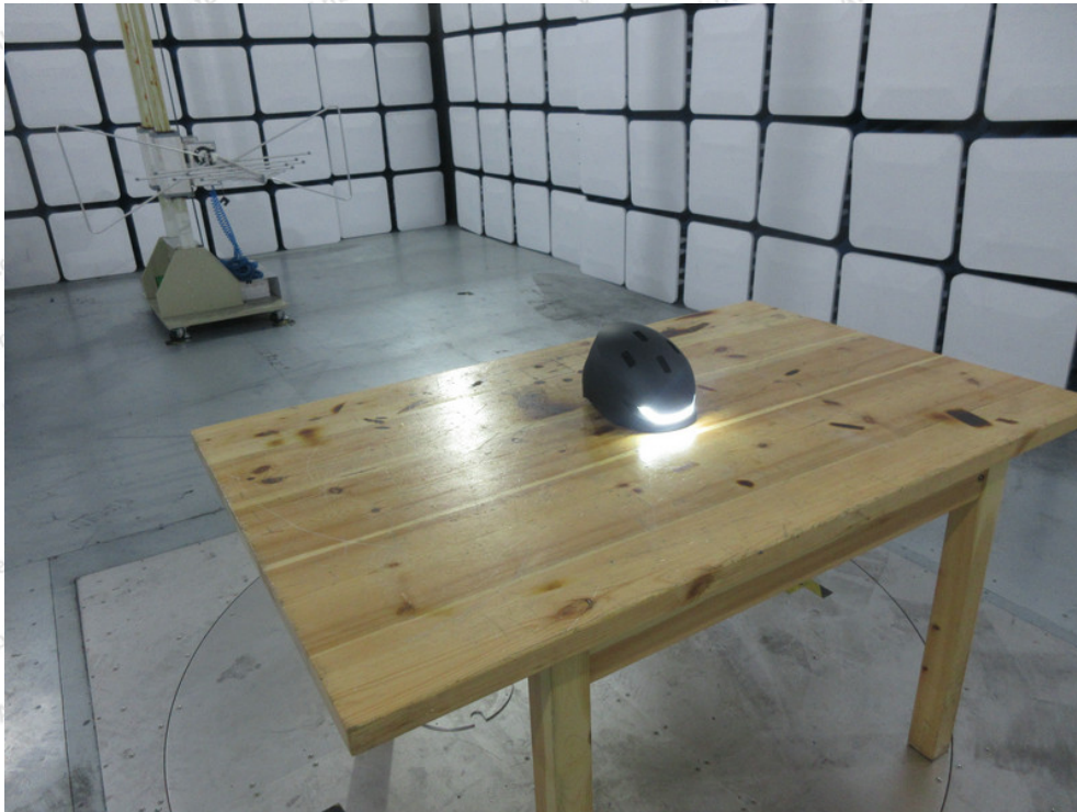
Photo of Radiation Emission Test
