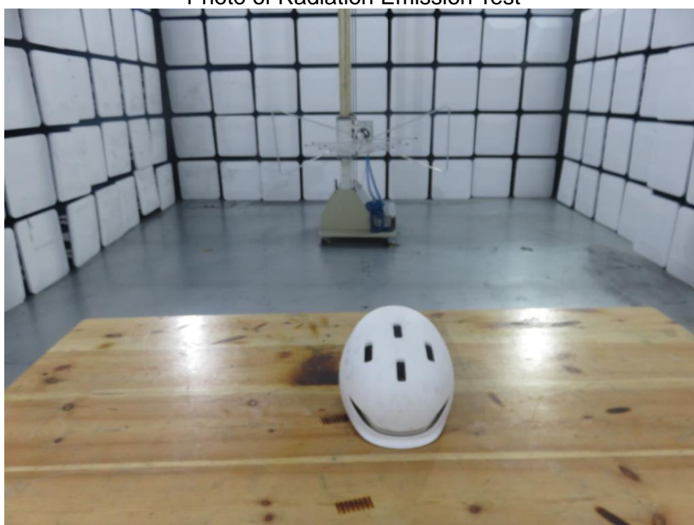
Photo of Radiation Emission Test
