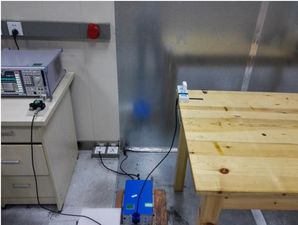
FCC RADIATED EMISSION TEST SETUP BELOW 1GHZ
