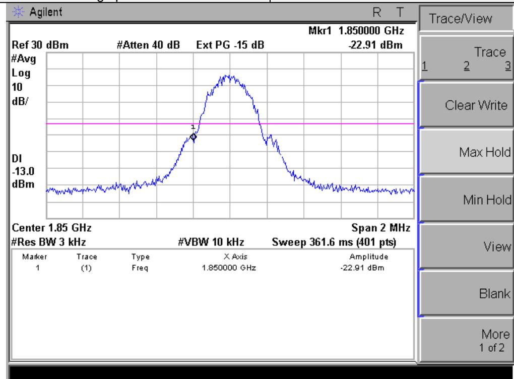
Note: Ext PG=Cable loss+10log(3.18/3)+Attenuator=4.75+0.25+10=15
