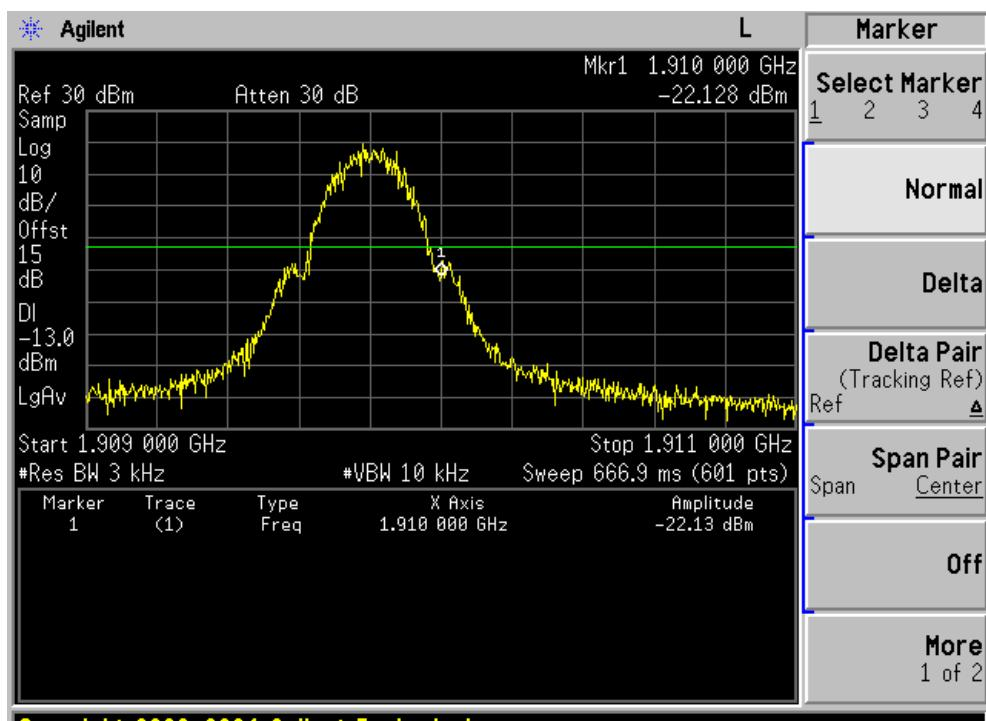
Conducted Band Edge plot on channel 9262
