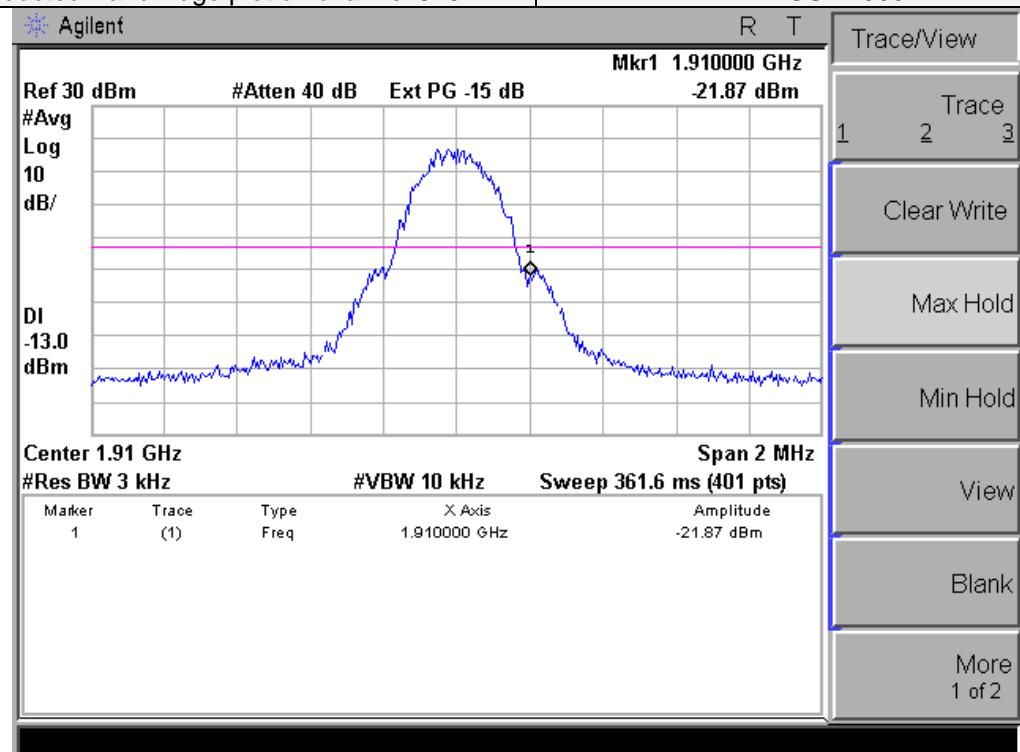
Note: Ext PG=Cable loss+10log(3.18/3)+Attenuator=4.75+0.25+10=15
