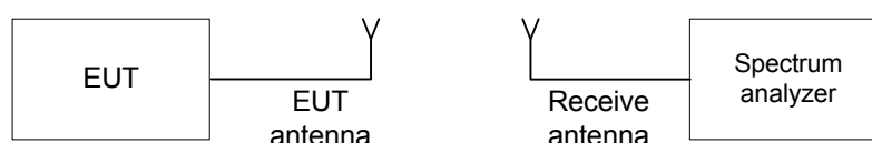
Figure 7.1.1 The 6 dB bandwidth test setup
