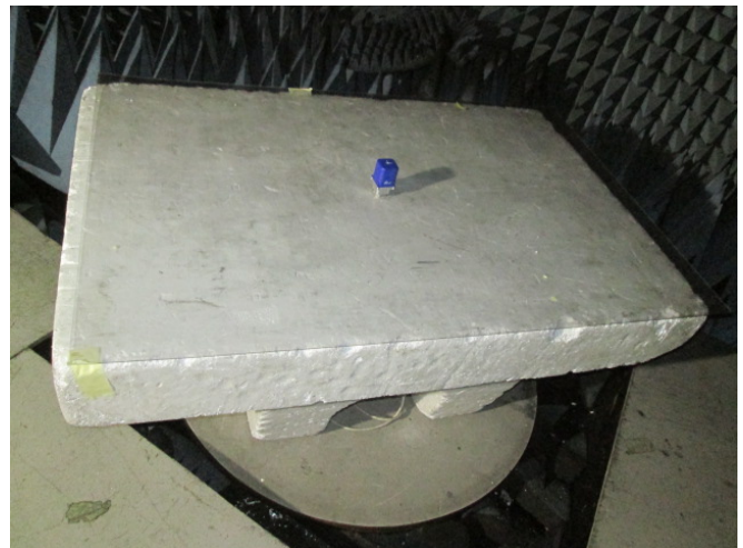
Photograph 8.1.1 Setup for radiated emission measurements
