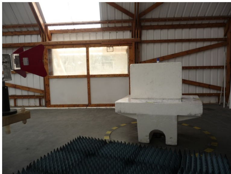
Photograph 8.1.2 Setup for radiated emission measurements
