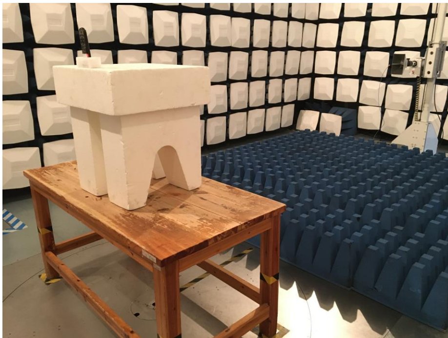
Test Setup For Radiated Emission (Above 1GHz)
