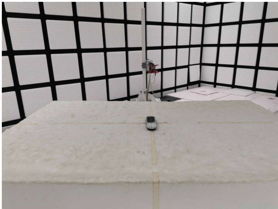
Radiated spurious emission Test Setup-2(Above 1GHz)
