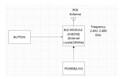
The HJH109 Ble remote control is mainly used for the control of household electric bed products to realize wireless control of the motor.
