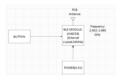
The HJH55B Ble remote control is mainly used for the control of household electric bed products to realize wireless control of the motor.
