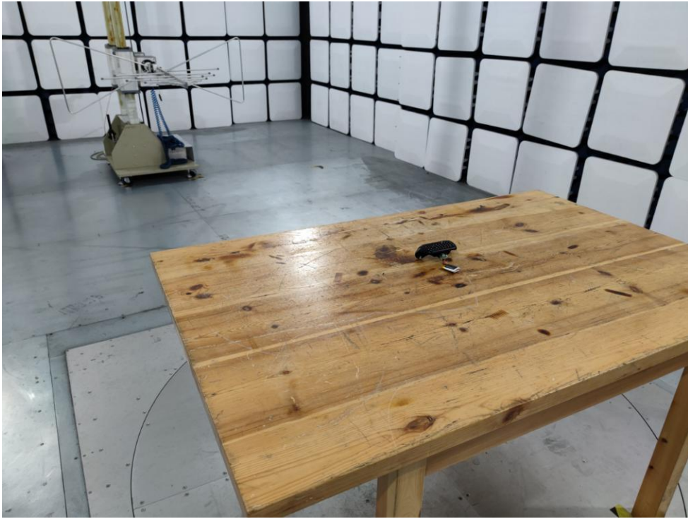
FCC ID: 2AJJC-TYX-586S Photo of Radiation Emission Test
