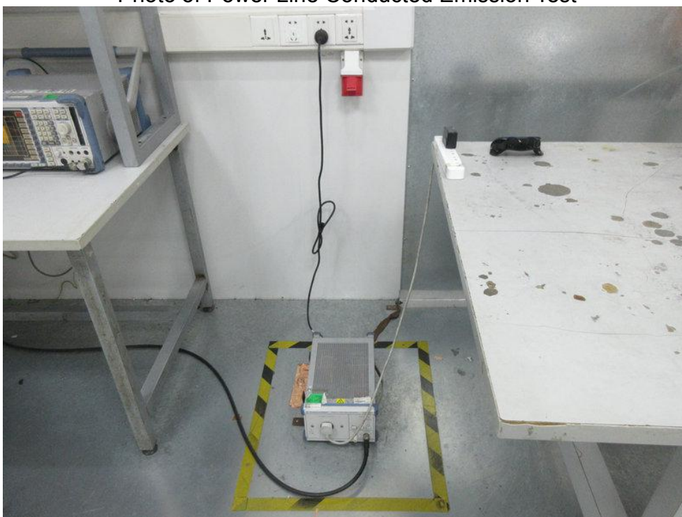
FCC ID: 2AJJC-TP4022 Photo of Power Line Conducted Emission Test
