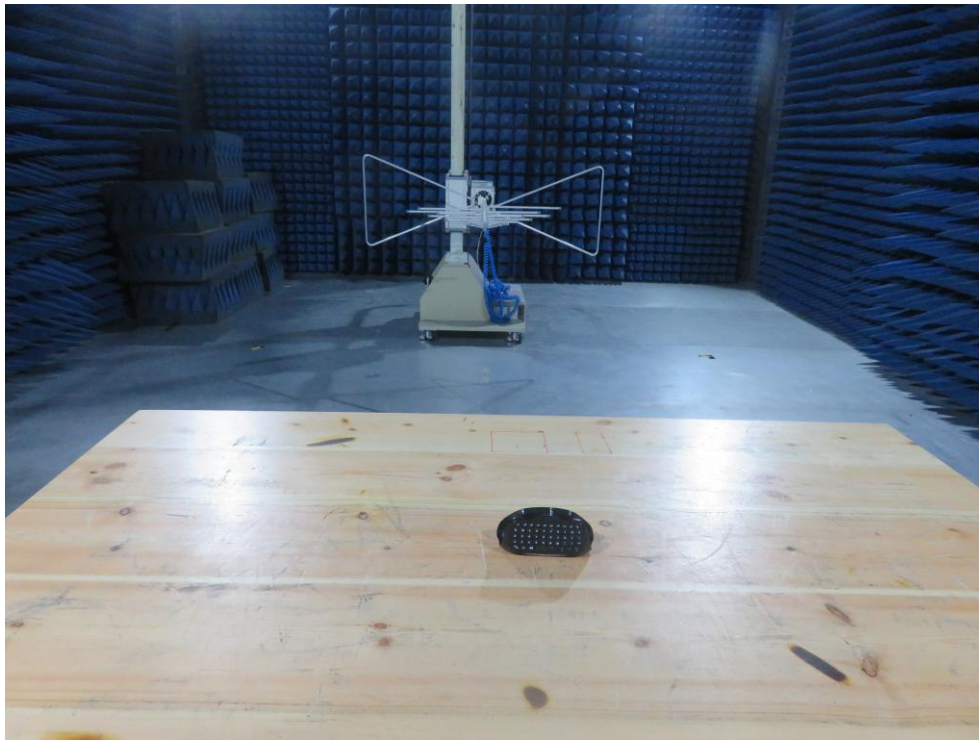
Photo of Radiation Emission Test
