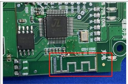
The antenna is PCB antenna. The best case gain of the antenna is -0.58 dBi.
