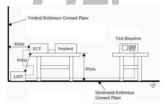
Remark: The EUT was connected to a 120VAC/ 60Hz power source.
