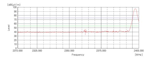
AV Detector: RBW: 1 MHz, VBW: 10 Hz (2 310 MHz - 2 390 MHz), Worst case (Low, Horizontal)
