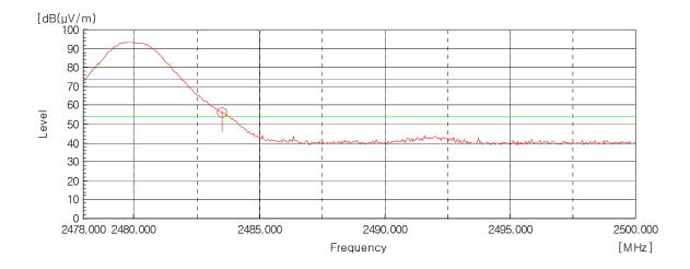
AV Detector: RBW: 1 MHz, VBW: 10 Hz (2 483.5 MHz - 2 500 MHz), Worst case (High, Horizontal)
