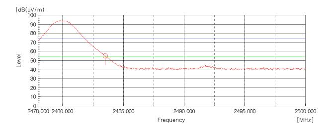
AV Detector: RBW: 1 MHz, VBW: 10 Hz (2 483.5 MHz - 2 500.0 MHz), Worst case (High, Vertical)
