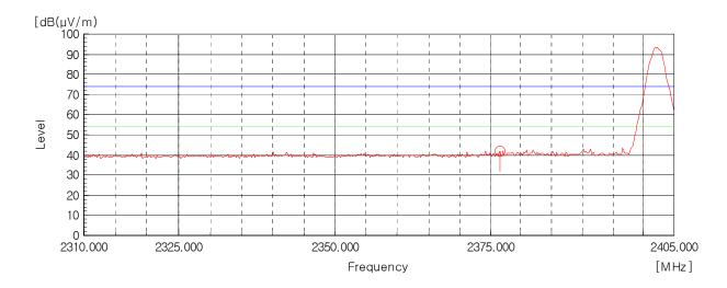
AV Detector: RBW: 1 MHz, VBW: 10 Hz (2 310 MHz - 2 390 MHz), Worst case (Low, Vertical)
